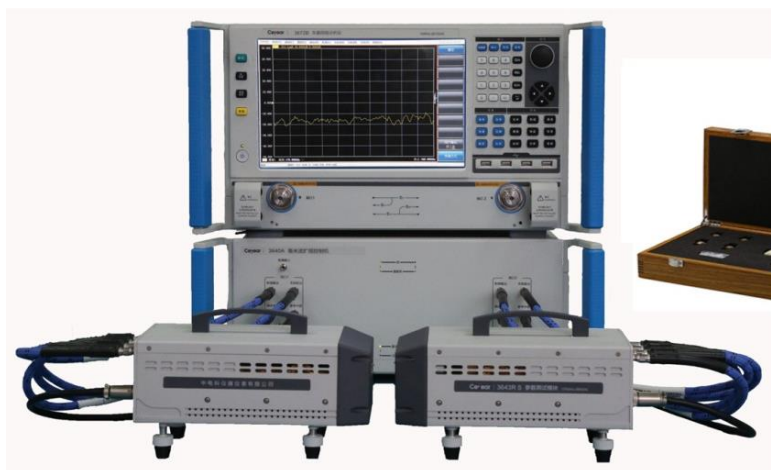
Fig. 2b Mm-wave and THz VNA System (Type-II: based on 2 ports VNA and controller)
